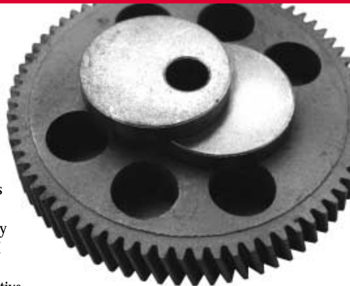
Designed for a leading manufacturer of dual-action electric hedge trimmers, this gear and cam assembly transfers the rotary motion of the motor into the reciprocating action of the trimmer blades.
