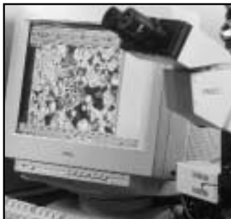
The Technology Center uses digital microphotography to analyze the microstructure of various P/M materials.
