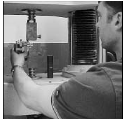
A sample is tested for tensile strength on the tensile testing machine in the MPP Technology Center.
