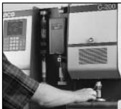
Carbon, oxygen, and nitrogen analysis is performed in the Instrument Lab of the Technology Center.
