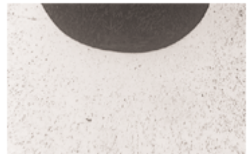
Pressed and sintered bevel gear root area after PCF (at 20X magnification)
