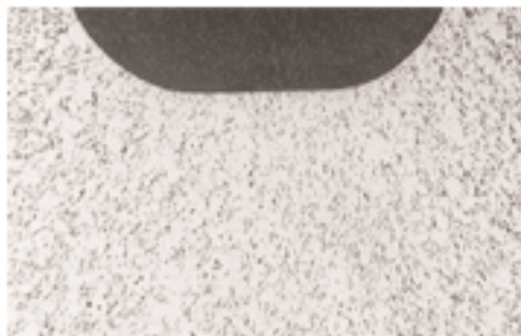
Pressed and sintered preform before PCF (at 20X magnification)
