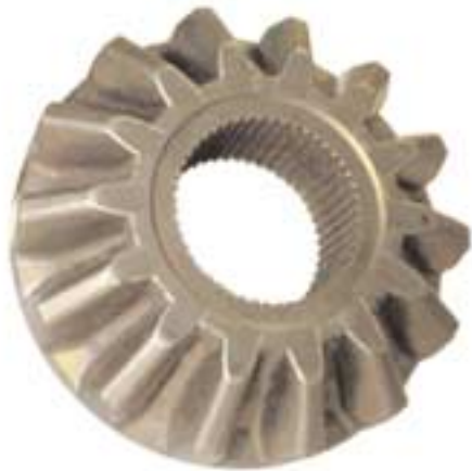
This fourteen-tooth bevel gear used in a high-performance garden tractor application was developed, using PCF technology, to replace a cut steel gear.
