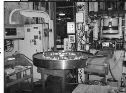
This computer-controlled 880-ton press will allow Ford Road to improve customer response time while producing more complex parts.
