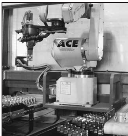
MPP's Anaheim and Washington Street Divisions have added robotics for part handling, turning, drilling, and inspection.
