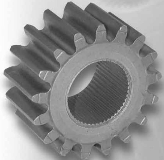
This seventeen-tooth PM spur gear used in a high-performance garden tractor application was developed to replace a cut steel gear. It is more economical and exhibits better fatigue strength than the cut gear.
